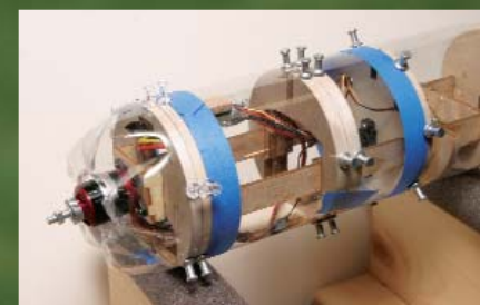
The Cermark motor is mounted on a small light-ply standoff to establish the appropriate thrust lines. I used push pins to position the screws that secure the plastic fuselage skins and cowl—all cut out of 2-liter soft-drink bottles.
